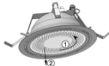
2. Remove reflector (for models with mounting brackets fixe.
