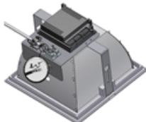
3.2.1. Put mains cable through strain relief and connect it to terminal block according to polarity shown (terminal block).
